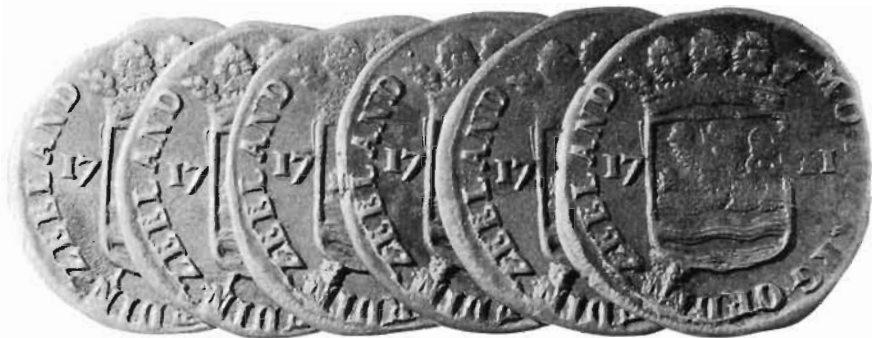
Plate 4 Progressional breakup of die at 7 O'clock.
