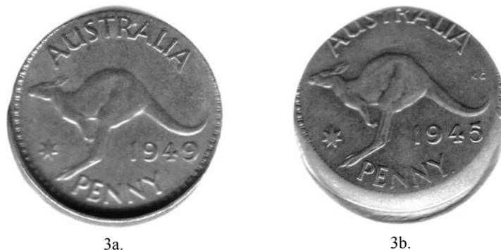
Figure 3. Off-centre error pennies. The cuppings indicate that the 1949 Melbourne mint penny had its reverse die uppermost in the coining press while the obverse die was on top for the 1945 Perth mint coin.
