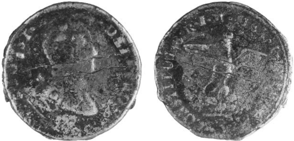
Figure 9. Obverse and reverse of a cast forgery of an 1822 Iturbide Empire Mexican 8 reales. Diameter 39–40mm, density 6.92gm/cc.
