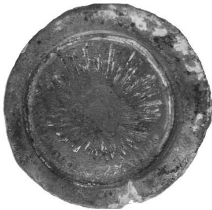
Figure 6. Mould for the reverse of an 18__ Mexican 8 reales forged coin (possibly the one shown in Figure 8).
