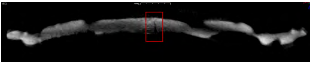
Figure 6a. 3D model of the Sirinos/Pyxis stater, ACANS inv. 07GS729; 6b. orthogonal cross section showing pores; 6c. orthogonal cross section showing crack.
